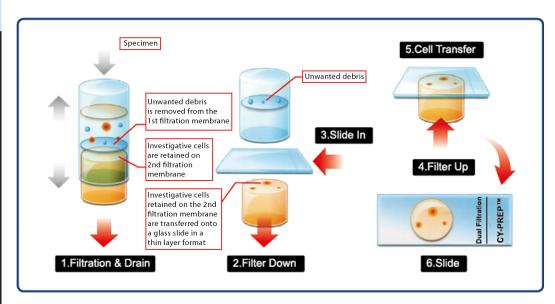
The CY-PREP® system automates every step of the slide preparation process. Slides are consistently prepared with excellent cellularity, morphology and distribution.
